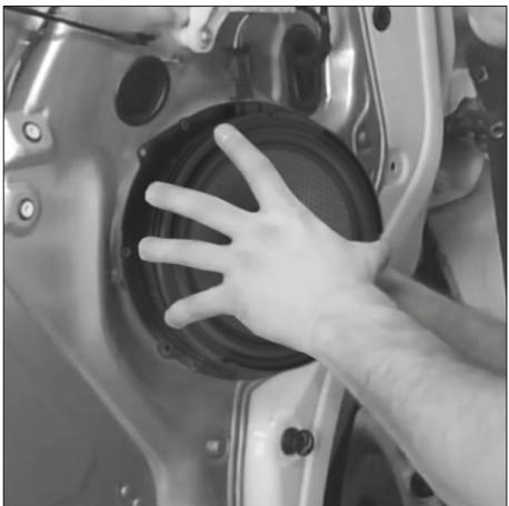
Put the new speaker in the opening after connecting it to the original cable.
