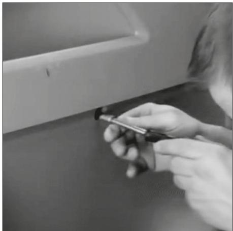
If there is a hand crank for the window, you must carefully remove it.
