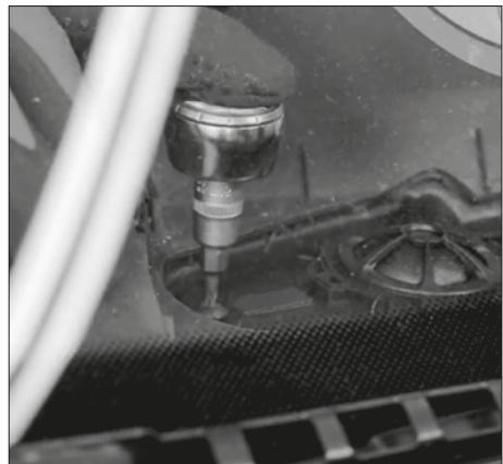
Fasten the new tweeter unit in the installation location with the original screws. Then build everything back again.
