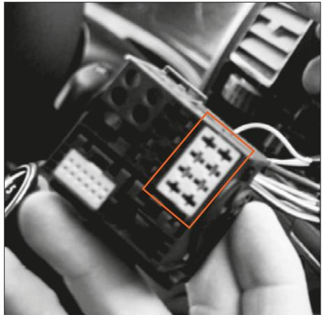
Unplug the vehicle's Quadlock connector from the car radio.
