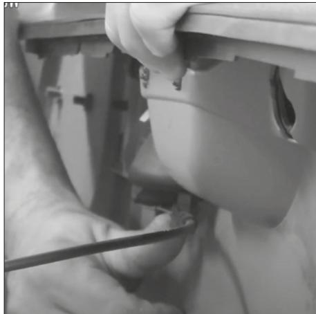
Remove the door handle release button by carefully unhooking it. If available, you still have to unplug the electrical window regulator plug.
