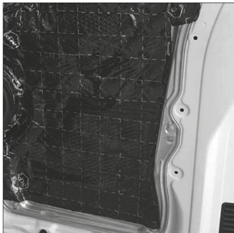
In order to achieve a better sound, it is recommended to dampen the doors with suitable damping materials such as aluminum-butyl insulating panels.
