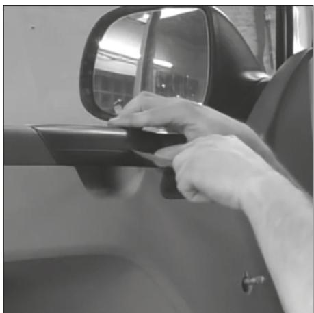
Remove the cover of the door handle at the top of the door panel.
