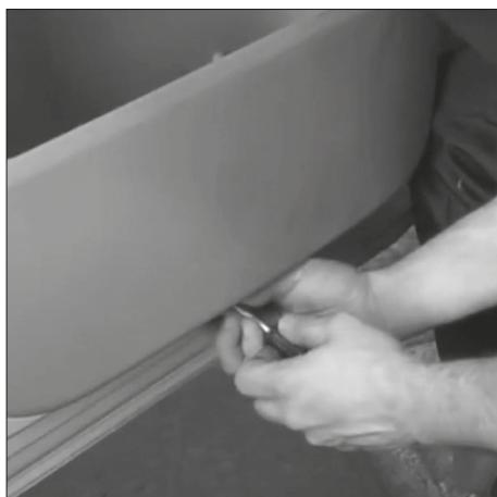
Loosen the three screws on the bottom of the door panel.
